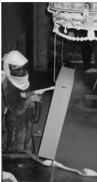
Powder application can be performed manually or with automated electrostatic spray guns.
