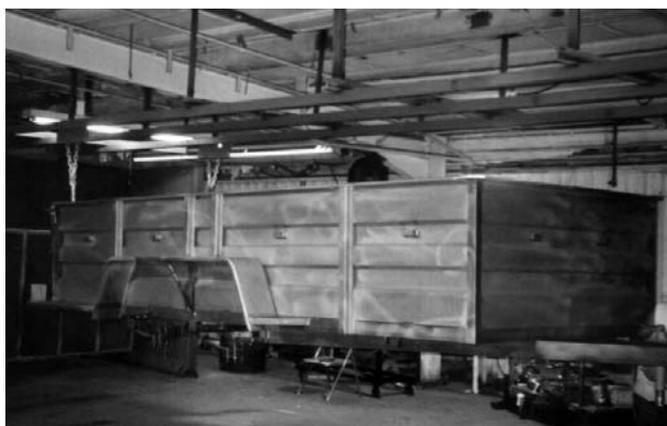
Entire trailer is powder coated. Part size is limited by curing oven.
